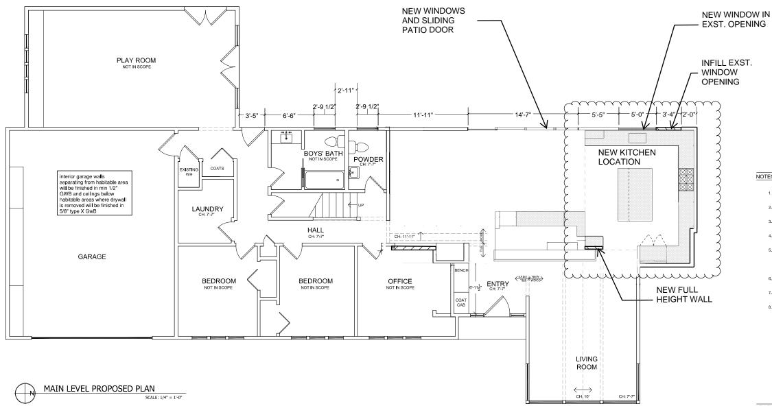
EXISTING EXTERIOR WALL LENGTH: 294'-6" LENGTH OF EXTERIOR WALL BEING ALTERED: 32'-4" PERCENTAGE OF EXTERIOR WALL BEING ALTERED: 11%
